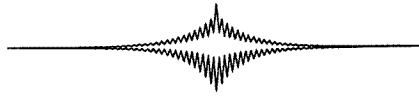
Figure 8. The calculated wavefunction amplitudes in the (\text{GaAs})_{76}\text{InAs}(001) superlattice, representing the InAs(GaAs) one-monolayer–host-crystal system. The upper curve corresponds to the electron state, while the lower curve represents the heavy-hole state.
